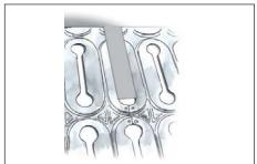
Install the cable and the flex pipe in the wall. The connection of the cable and the thermostat must be carried out by an authorised electrician.
